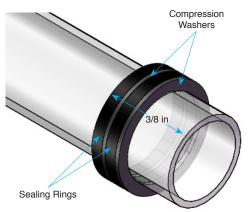
Figure 3: Quartz Tube Seal Assembly Detail
